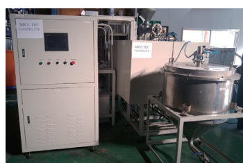
Microwave sintering furnace
